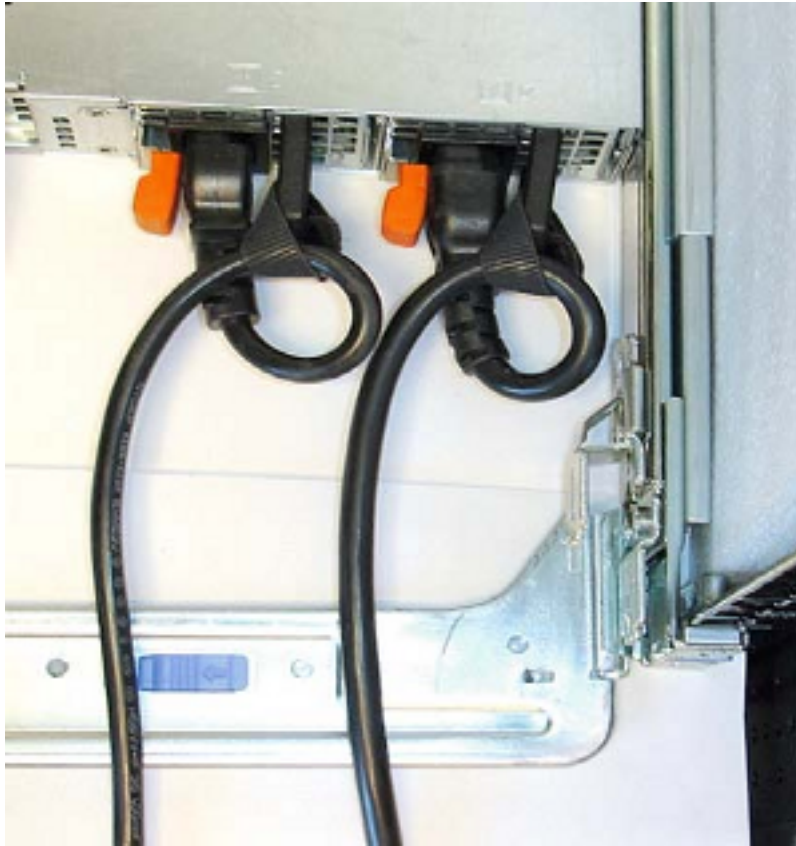
Figure 23: Proper PSU Cabling
