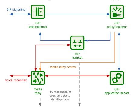
Figure 2: SIP and Media Relay Components
