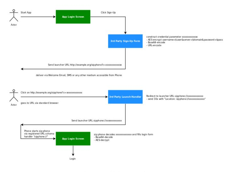
Figure 143: Provisioning Push Workflow
