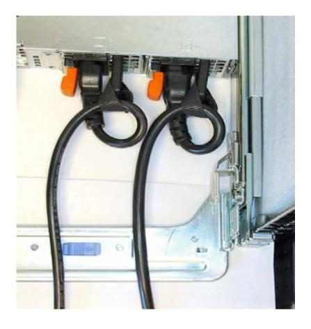
Figure 12: Proper PSU Cabling
