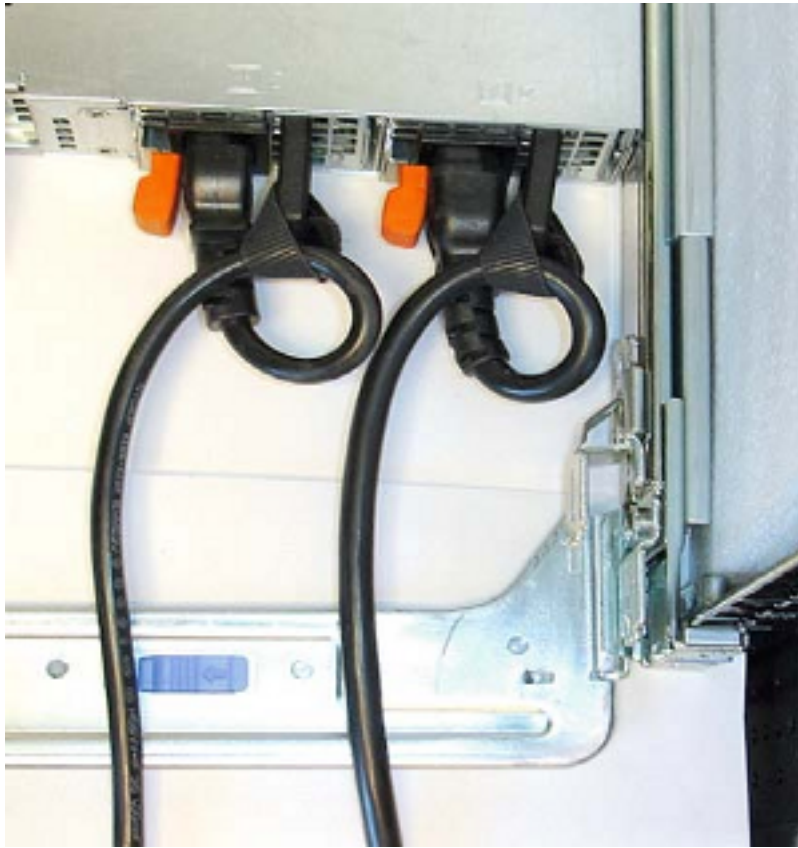
Figure 12: Proper PSU Cabling
