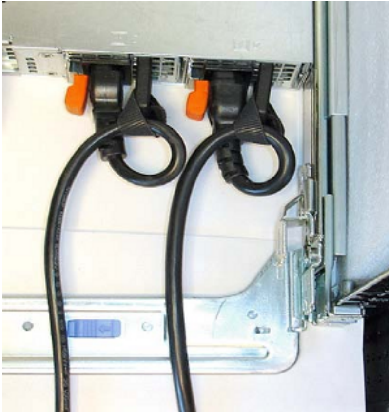
Figure 12: Proper PSU Cabling
