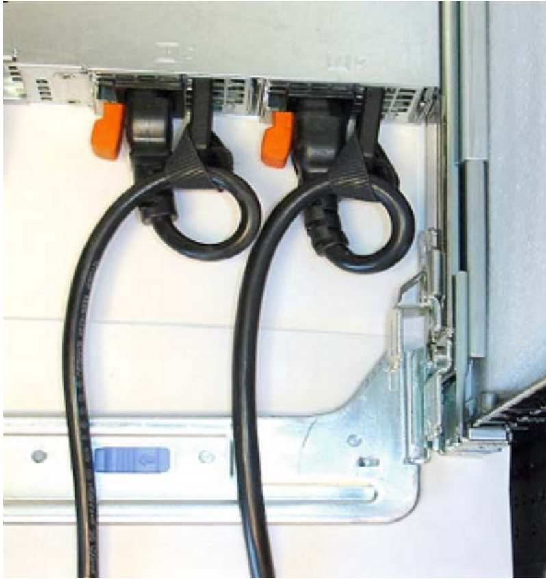
Figure 12: Proper PSU Cabling
