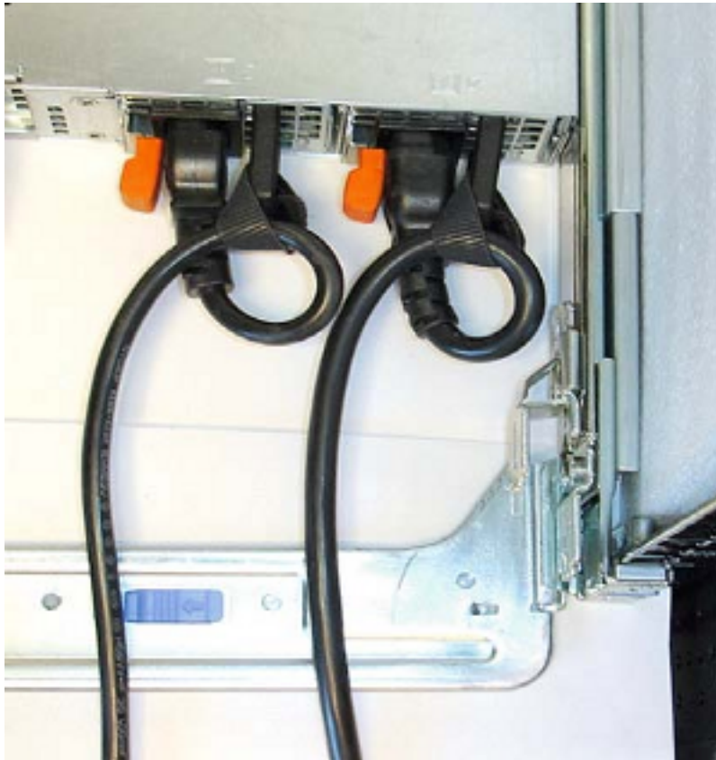
Figure 12: Proper PSU Cabling
