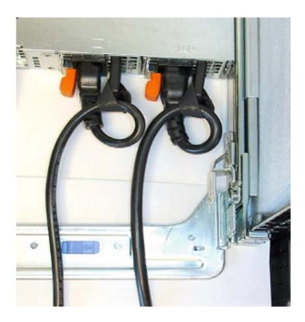
Figure 12: Proper PSU Cabling
