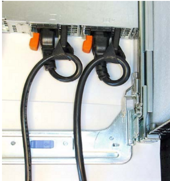
Figure 10. Proper PSU Cabling
