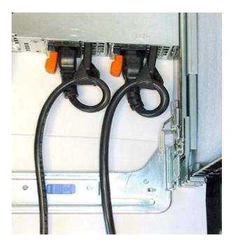
Figure 9. Proper PSU Cabling
