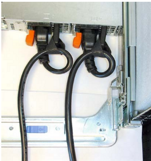
Figure 9. Proper PSU Cabling
