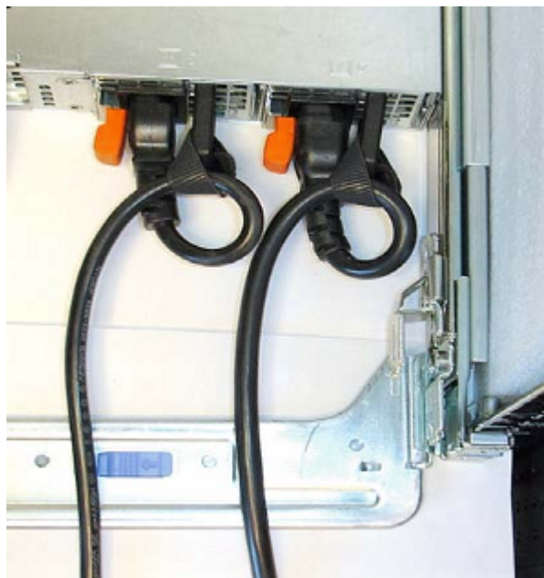
Figure 9. Proper PSU Cabling
